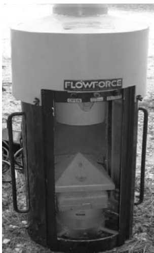
Figure 1. Feed sensor used to calculate feed weight
